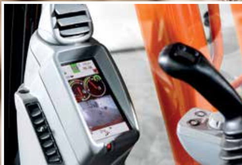
The LCD monitor shows the machine's status and settings.
